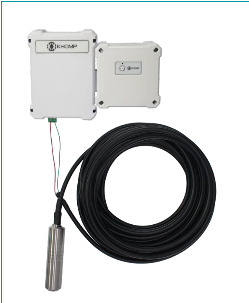
Caption: This image presents a Liquid Level Sensor connected to the modular EM C104 extension unit. The system is integrated into the IEEE 802.15.4 Endpoint in order to provide the ITG gateway with wireless data transmission.
